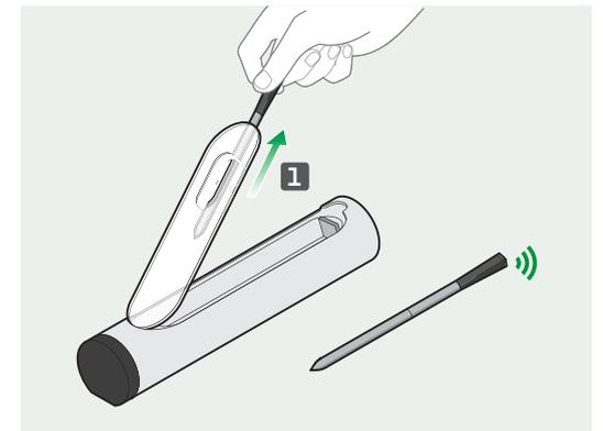
**4.** Open the charger and extract the probe. When you remove the probe from the charger, the LED flashes green indicating the charger is connected to the probe.
