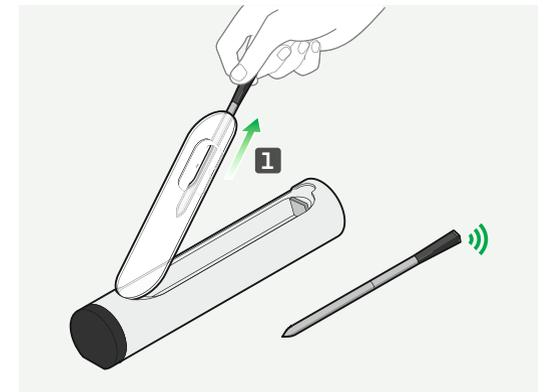
**4.** Open the charger and remove the probe. When you remove the probe from the charger, the LED flashes green indicating the charger is connected to the probe.
