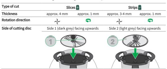
The thickness is set using the rotation direction.
